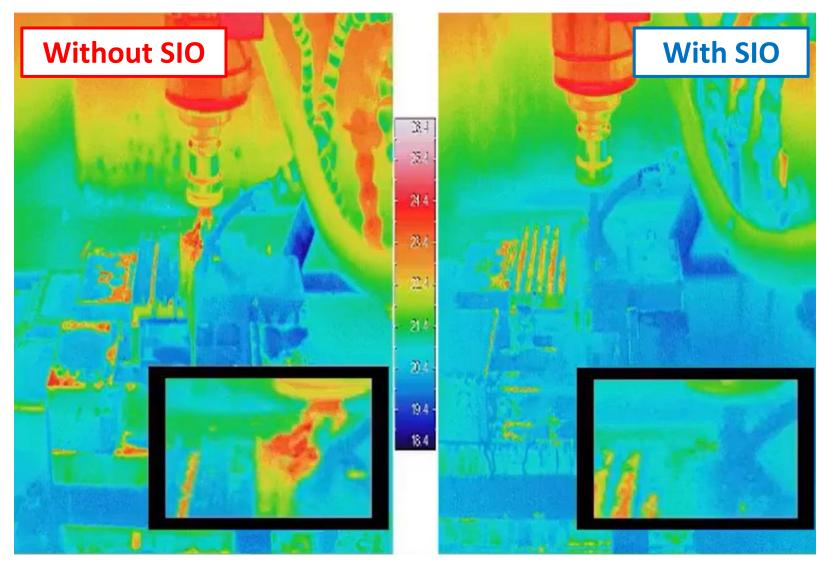
• Improved cooling performance of metalworking fluid after passing through SIO
