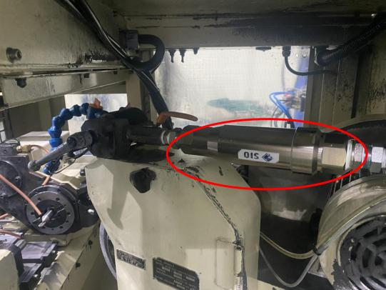
Supply: 110-130 LPM @ 3-5 bar: SIO 1 inch before manifold
